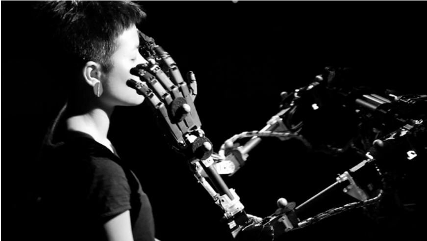
Fig. 7 The Blind Robot (Louis Philippe Demers) consists of a set of two-mechanical arms mounted onto a base and bolted to a table. Visitors are invited to interact with the robot by sitting in a chair as the robot delicately explores the sitter's face and upper body in a manner that recalls how blind humans supposedly use touch to recognize persons or objects. (Photo by Louis Philippe Demers)
