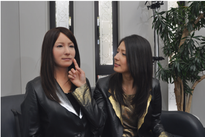
Fig. 5 Android robot, Geminoid F ( left Geminoid F, right original person )
