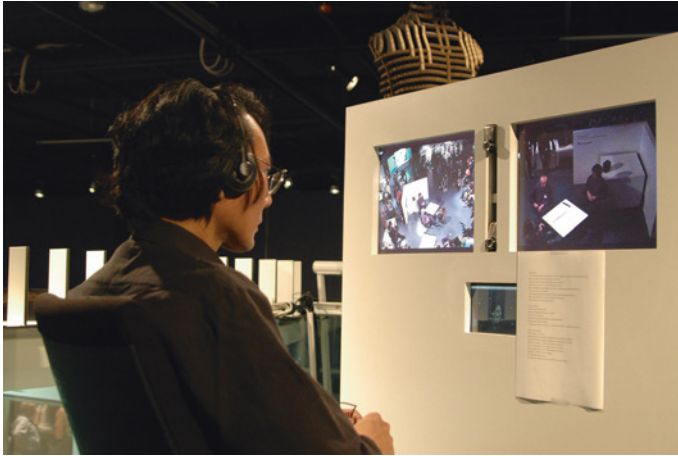
Fig. 2 The tele-operation console of Geminoid HI-2
