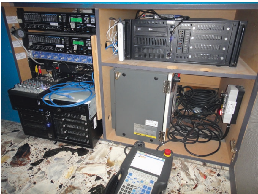
Fig. 6 Various computing and other hardware equipment used by the Articulated Head during its two year run at the Powerhouse Museum—just before being dismantled permanently at the end of the project. The bulk of the robot software was run on two high-end servers, one running a flavor of Linux and the other Microsoft Windows, respectively. It was a nostalgic moment for the team taking out parts of the robot, reminiscent of the iconic scene from Kubrick’s classic movie “2001: A Space Odyssey”. Image by Damith Herath
