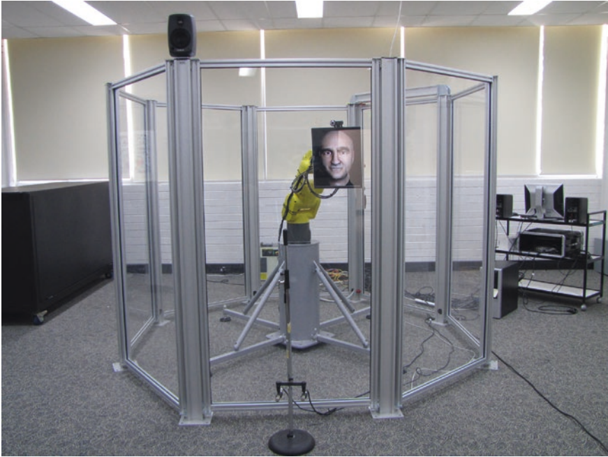
Fig. 4 Articulated Head inside its new aesthetically designed mobile enclosure. Image by Damith Herath
