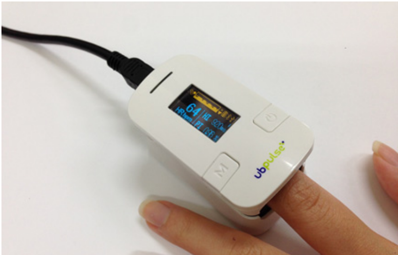
Fig. 2 A commercial PPG sensor used in the experiment [5]
