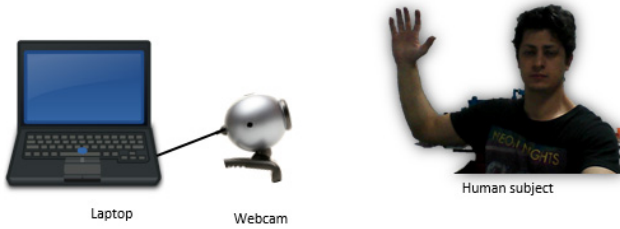
Fig. 1 Conceptual diagram of webcam based motion tracker
