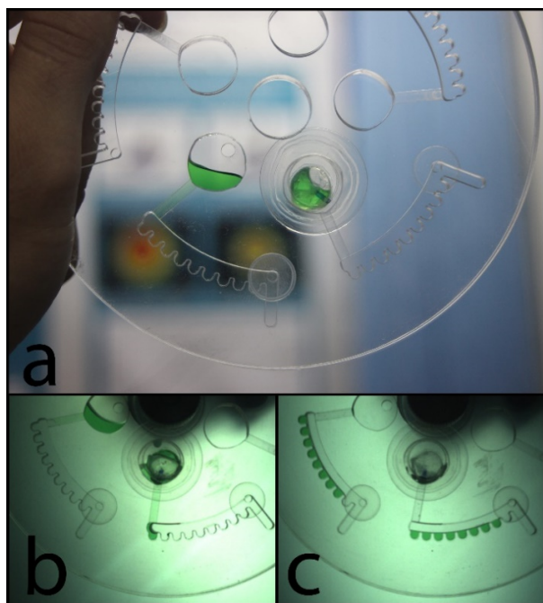
Fig. 2 (a) The liquid sample was pipetted into the source chamber of the left microfluidic unit, while the right microfluidic unit was equipped with a reagent storage device i.e., a liquid-filled bubble with a latex membrane. (b) The bubble was burst with the help of an external mechanical force. (c) The disc was spun and the liquids were transferred into the metering chambers.
