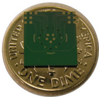
Fig. 1 Multi-analyte biochip (MAB) consists of multiple working and reference electrodes.
