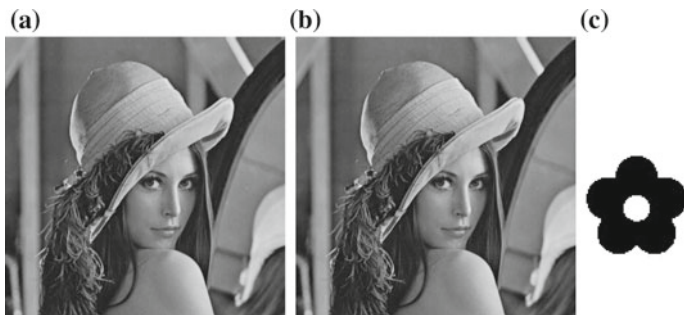
Fig. 2 a Original image. b Watermarked image with t = 1.5 (PSNR = 56.1787 dB). c Extracted watermark (NC = 1)
