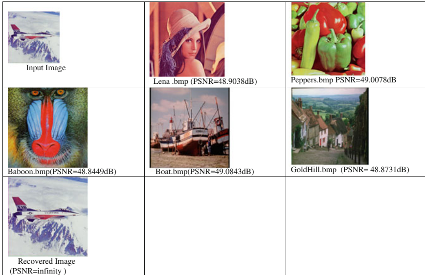
Fig. 4 Experimental results of the proposed scheme for color images with no expansion in cover images
