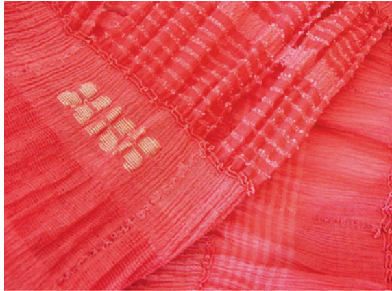
Fig. 5 Songket textile, silk and metallic yarns woven by Suzanne Stankard. Sections of warp are drawn together by twisting of floating high-twist weft yarns, which caused a vertical line of texture (160 × 30 cm) [4]
