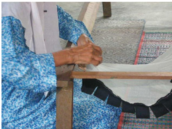
Fig. 5 The process of stretching the base fabric onto the pemidang (Source Rose Dahlina Rusli)
