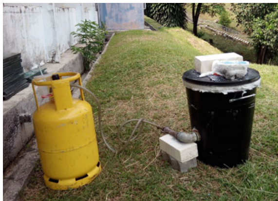
Fig. 4 Firing process using the kiln built from a dustbin container
