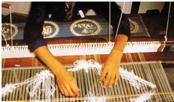
Fig. 1 Weaving songket using lashes of ikat butang for making the songket motifs, where the gold metallic yarns are inserted between the warps and firmed with plain weaves
