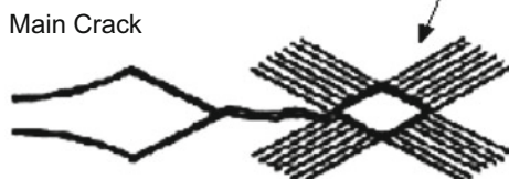
Fig. 7.2 Striations on the tensile-fracture surface of a hydrogen-charged iron single crystal specimen. The lower illustration is a schematic STM view showing a microcrack formed at the intersection of striations (Terasaki et al. [3])
