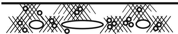
Fig. 10.7 Illustration of the HESIV model for the creation and clustering of vacancies forming microcracks in strain-concentrated area close to a barrier for slip extension
