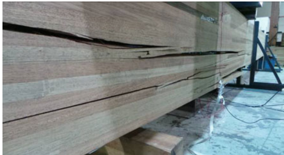
Fig. 7 Failure mode of Mengkulang glulam, the beam failed in ductile manner
