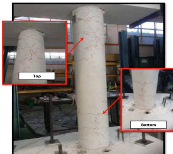
Fig. 3 Damages of the first column before retrofitting
