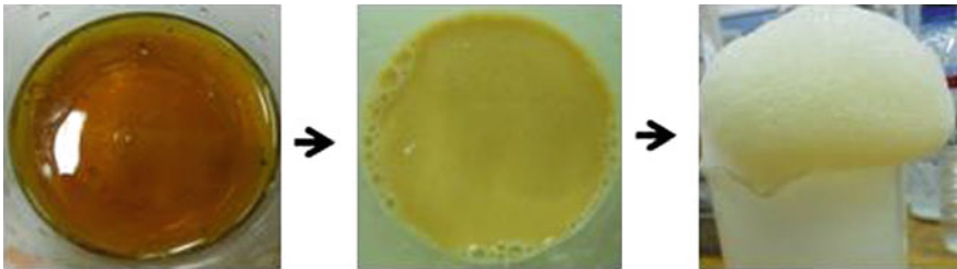
Fig. 2 The transition of used cooking oil begin formulated become foam
