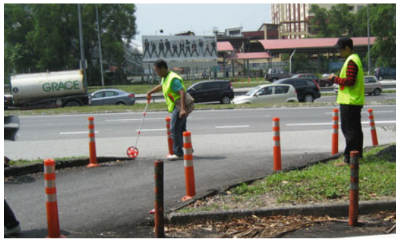
Fig. 7 Measure the geometrical characteristic parameters using roller meter
