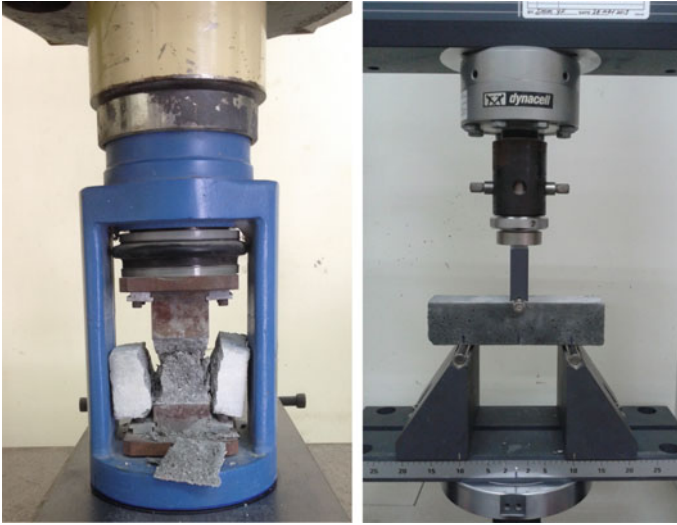
Fig. 2 Compressive and flexural testing of FGM
