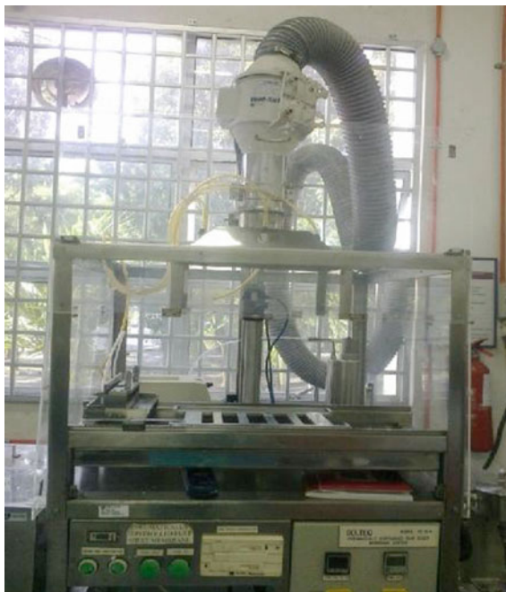
Fig. 2 Flat sheet membrane casting machine
