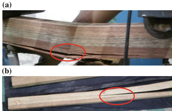
Fig. 8 Failure mode characteristics of untreated Mengkulang glulam under bending: a simple tension, b horizontal shear
