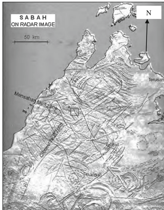
Fig. 3 Kundasang ( square ) located at the intersection of two major active faults, the Mensaban and Crocker Fault Zones ( source from [2])
