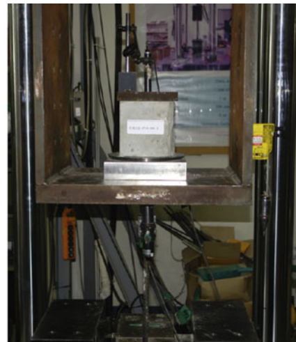
Fig. 2 Cube pullout specimens schematic and detailed test setup [2]
