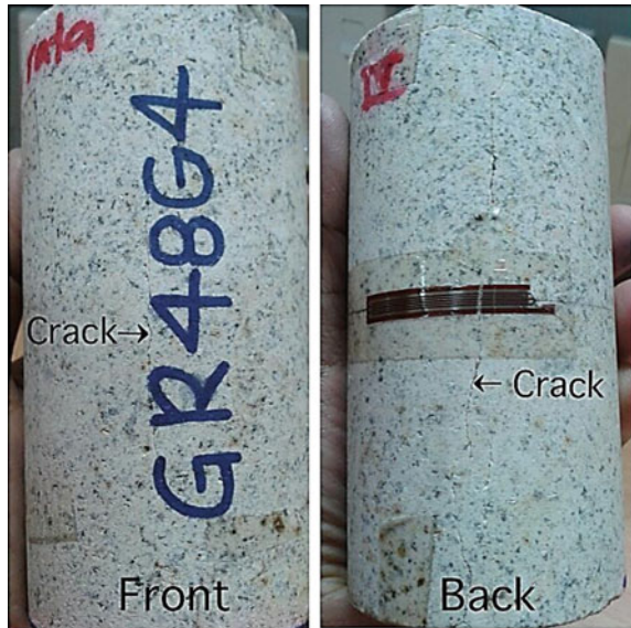
Fig. 8 Crack presence on specimen surface
