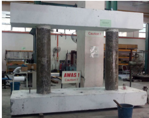
Fig. 5 Columns' surface was coated with Primer Epoxy Resin before wrapping with CFRP
