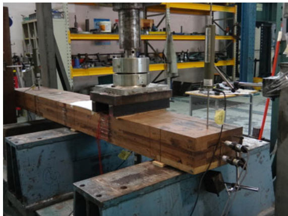
Fig. 1 Flexural fatigue test setup at rail seat of sleepers
