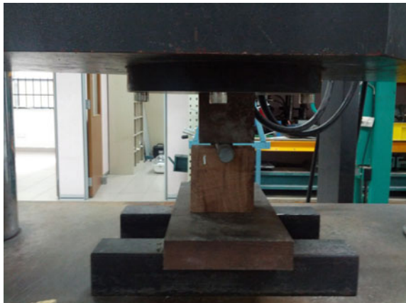
Fig. 4 The arrangement for dowel-bearing test procedure using UTM machine
