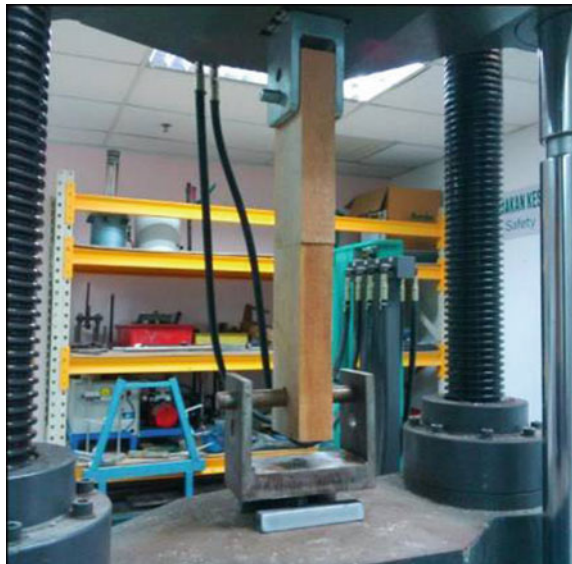
Fig. 5 Test setup for tensile test on timber jointed with bonded-in rod
