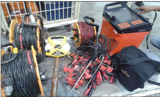
Fig. 4 Seismic refraction survey equipments
