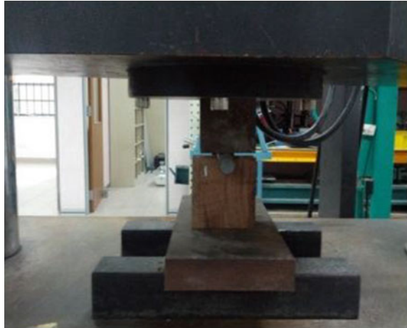
Fig. 3 The arrangement for dowel-bearing test procedure using UTM Machine
