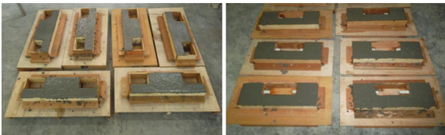
Fig. 9 Specimens casting process
