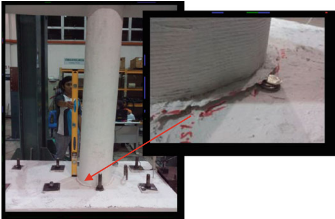
Fig. 11 Failure of the joint at pulling direction after \pm 2.25\% drift
