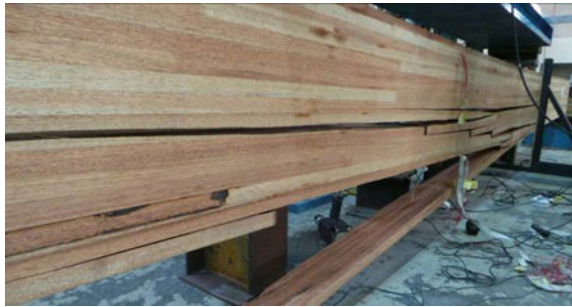
Fig. 6 Failure mode of Mengkulang glulam, failure start at tension zone
