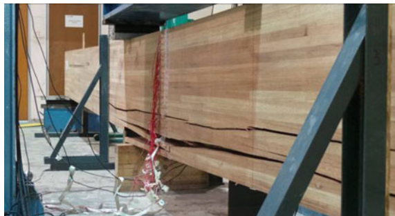
Fig. 4 Failure mode of Mengkulang glulam, failed in timber
