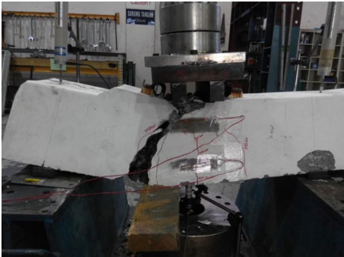
Fig. 11 Sample after failure post-fatigue test
