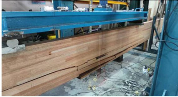
Fig. 5 Failure mode of Mengkulang glulam, the timber failure at finger joint (indicates good manufacturing process)
