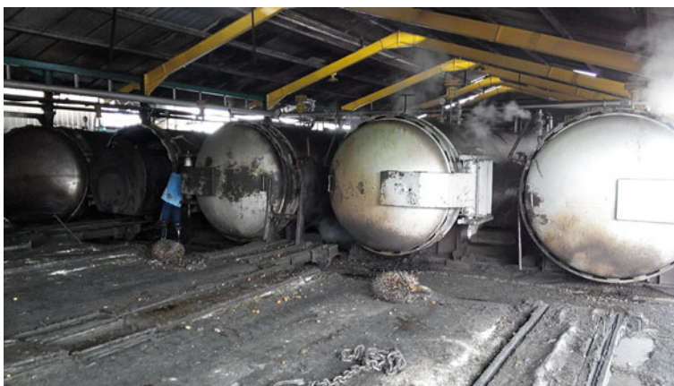
Fig. 3 Horizontal cylindrical autoclaves
