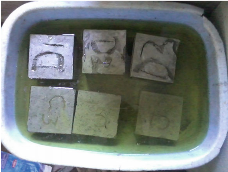
Fig. 3 Curing of S/S mortar blocks
