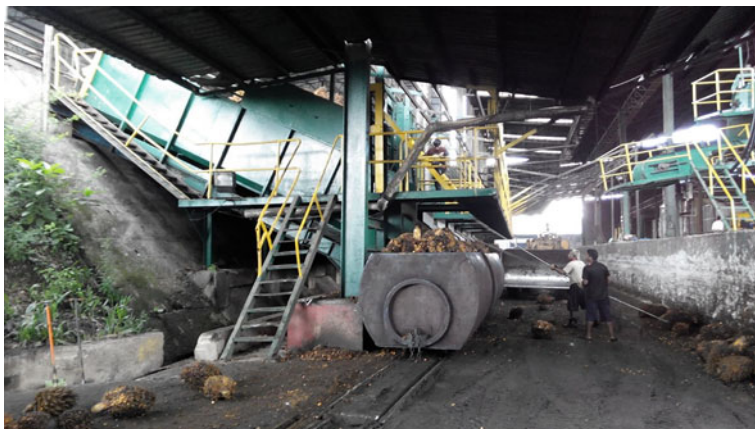
Fig. 2 Fresh Fruit Bunch ramp
