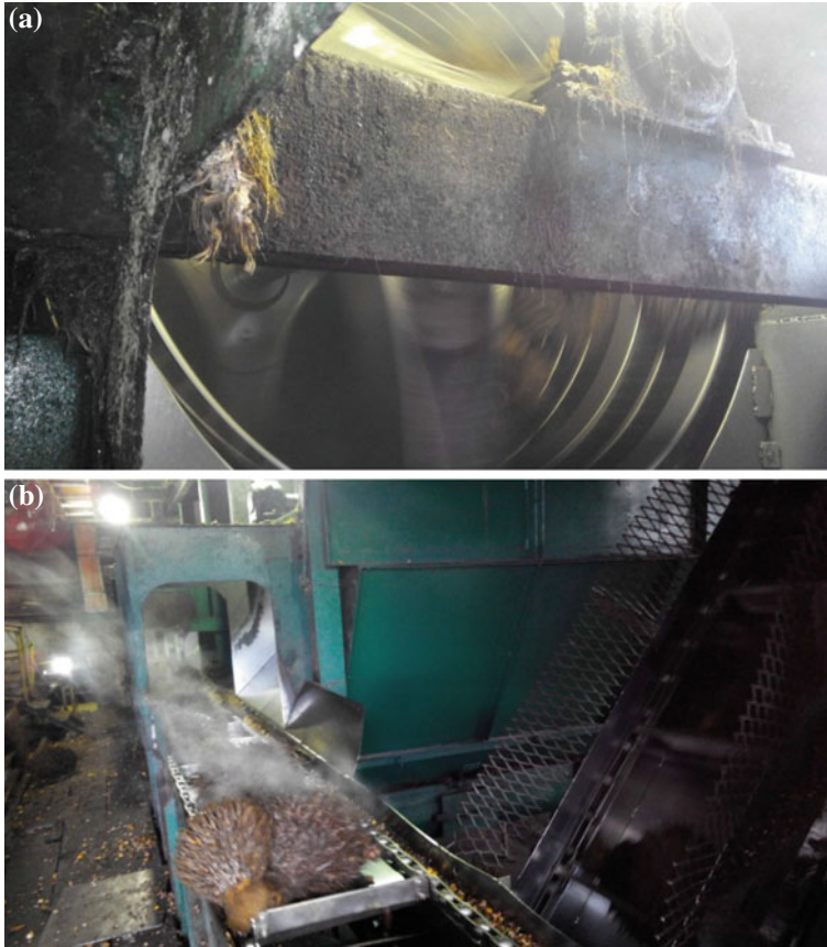
Fig. 4 Revolving slated steel drum for fruit recovery (a) and palm oil drum strippers (b)
