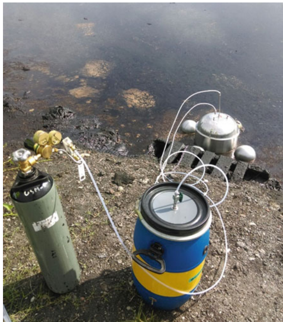
Fig. 1 Odour sampling at an effluent pond using flux hood and vacuum chamber
