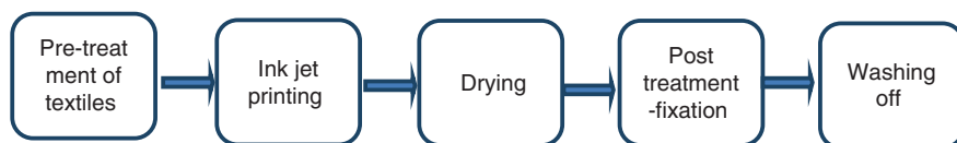
Fig. 6 Digital printing process of textiles (Chavan 1996)
