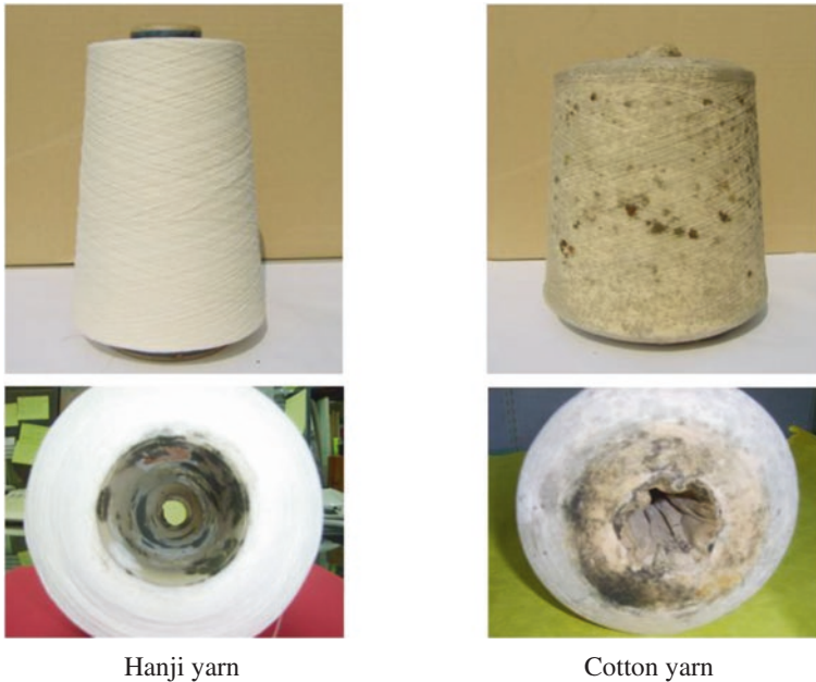
Fig. 4 Ssang-Young's antimicrobial activity testing results comparing Hanji and cotton yarn left at 77 °F with 80 % humidity for one month in April (Ssang-Young 2015)
