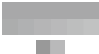
Fig. 20.2 The arrangement of samples in the grayscale method
