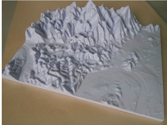
Fig. 44.4 Photograph of the physical model of NSDTF-DEM printed by Matrix 300A
