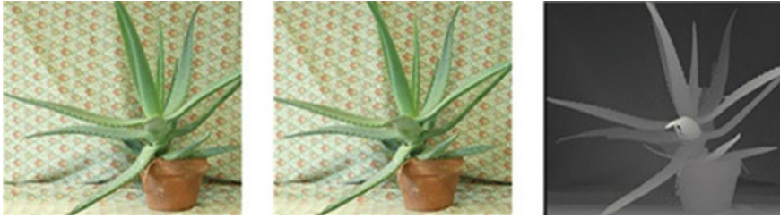
Fig. 3 Disparity map image obtained using a stereo camera
