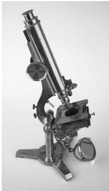
Figure 3. Darwin's achromatic microscope, made by James Smith in 1846. (By kind permission of the Whipple Museum, Cambridge.)
