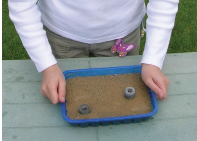
Figure 3. Liquefaction in a sand tray. (© Peter Kennett)
