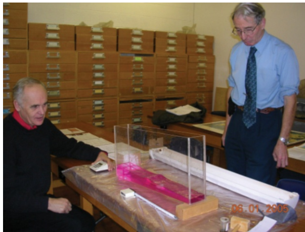
Figure 5. Timing a 'tsunami' in a wave tank. (© Peter Kennett)
