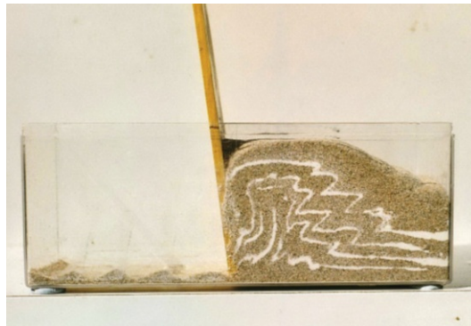
Figure 1. Folding and faulting in an empty chocolate box. (© Peter Kennett)
