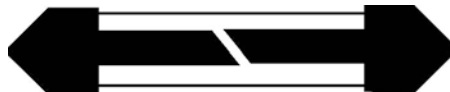
Fig. 7.3 This schematic image of a glow lamp clearly shows a gap between the two electrodes. Yet Birgit notices it for a first time, with surprise, only after having tried for a long time to make the experiment work – though it was not because of the gap, which is a constituent and necessary feature of this device.
