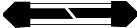
Fig. 7.3 This schematic image of a glow lamp clearly shows a gap between the two electrodes. Yet Birgit notices it for a first time, with surprise, only after having tried for a long time to make the experiment work – though it was not because of the gap, which is a constituent and necessary feature of this device.
