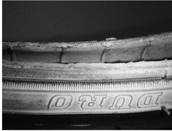
Fig. 7.1 This photograph of a tire clearly shows the coiled wire bead on the back part and the way the tire is shaped to fit and hold onto the steel rim. In the episode recounted here, the tear appeared just below the wire.
