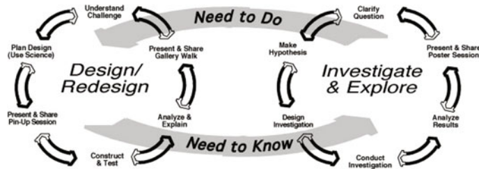
Figure 2. The Learning By Design™ design/inquiry process model emphasized a dialog between strategies associated with scientific investigations and with engineering design (Kolodner, Gray, & Fasse, 2003).
