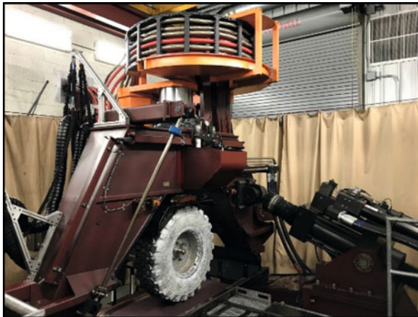
Fig. 23.12 MTS FlatTrac LTR System with MPT 81 Tire Installed
