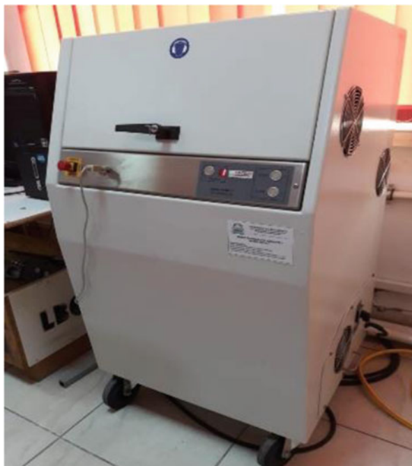
Fig. 12.1 Fritsch Pulverisette 4 vario-planetary mill (UCV laboratory)
