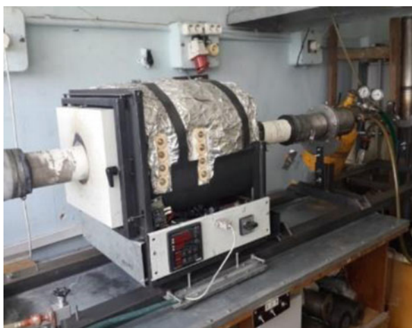
Fig. 9.3 Rotary tube furnace for synthesis of nanopowders
