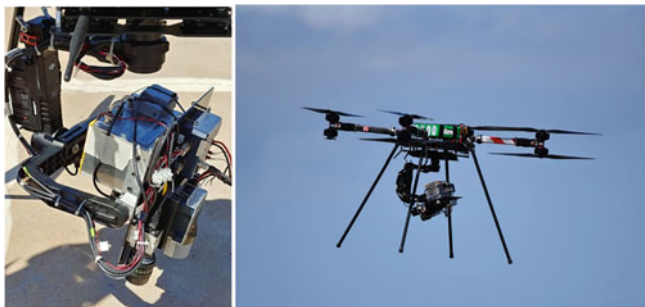
Fig. 17.11 (Left) – Photograph of the LiDAR system integrated and balanced onto a 3 axis Ronin Gimbal. (Right) – Complete system successfully operating in-flight
