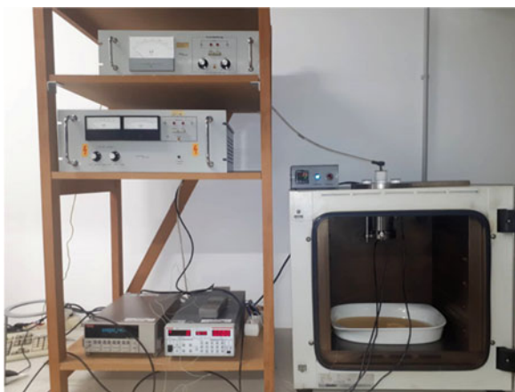
Fig. 3.5 Photographs of the developed corona triode. In the left, the single components can be observed and, in the right, the assembled system
