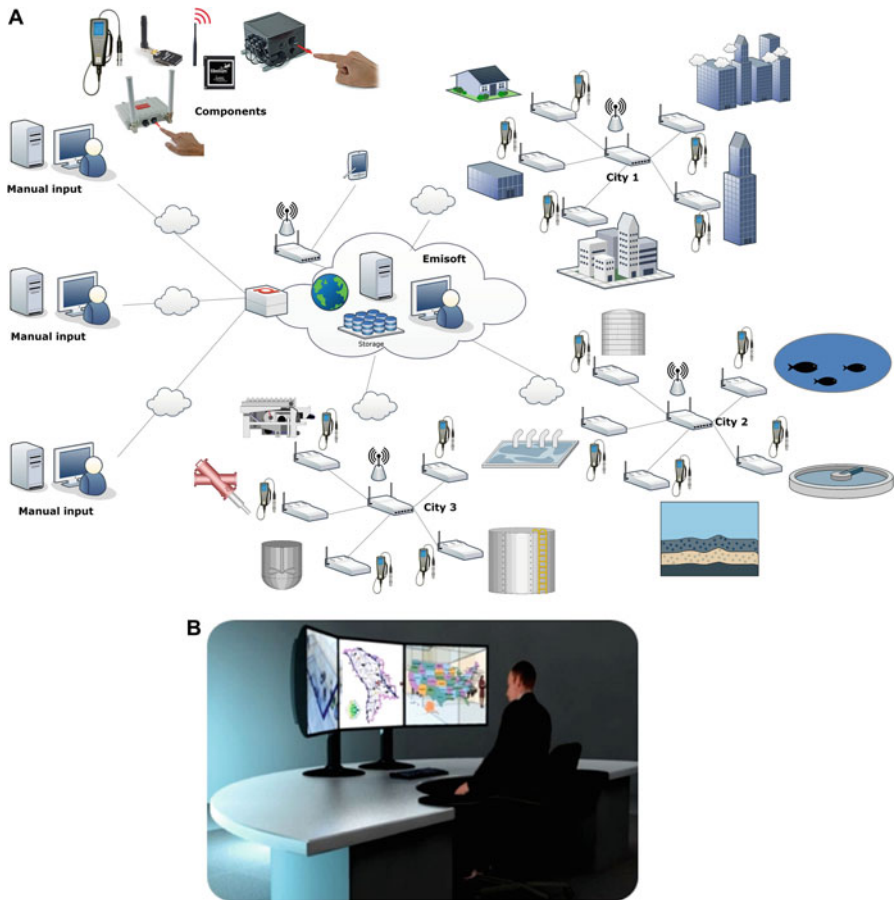
Fig. 1.3 (a) Distributed sensor system using remote, wireless data transmission and data gathering, (b) Artist's rendition of CILM-EDS unit
