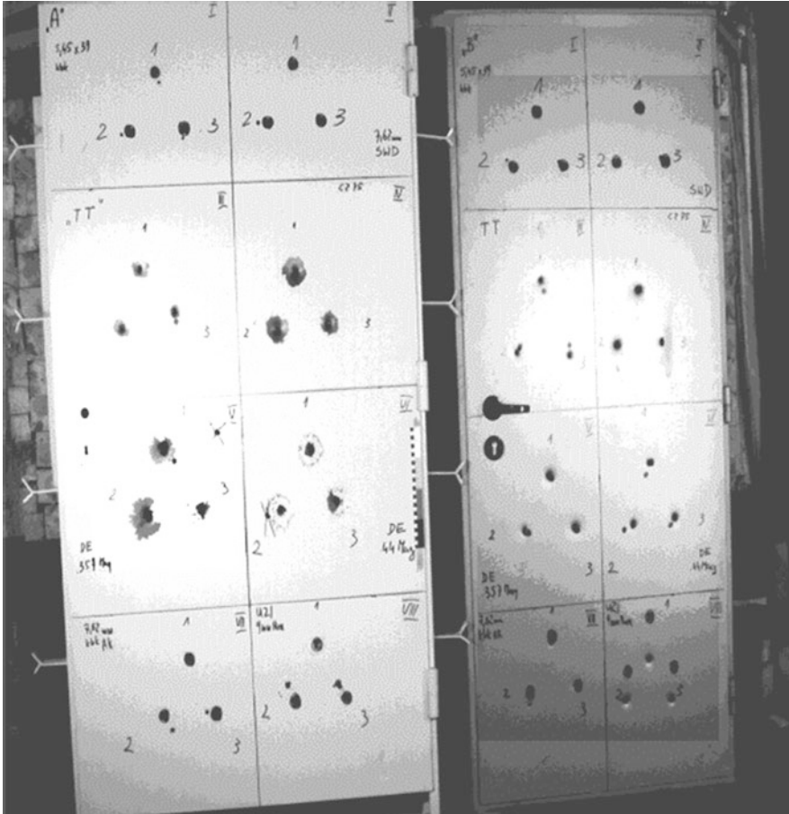
Fig. 18.1 Protective steel doors, type A (left) and B (right), following laboratory perforation tests
