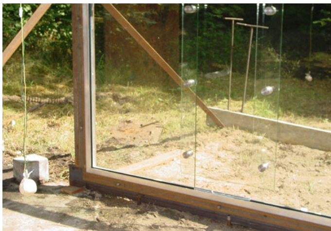
Fig. 18.10 The cash desk window structure on the testing stand. The spherical charge of the explosive is visible
