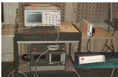
Fig. 18.21 Diagram of measurement circuit used to record pressure and displacement as a function of time. 1 – tested pane or protective window, 2 – PSx-20 sensor for displacement measurement and M102 sensor for pressure measurement, 3 – measurement amplifiers, 4 – V-STORE recorder, 5 – Infiniium digital oscilloscope – see Fig. 18.11
