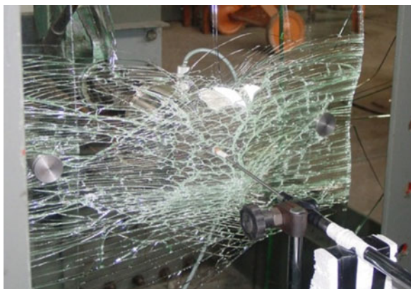
Fig. 18.6 Cracked panes of the cash desk window at maximum static load 2042 N – view from the side where the load was applied
