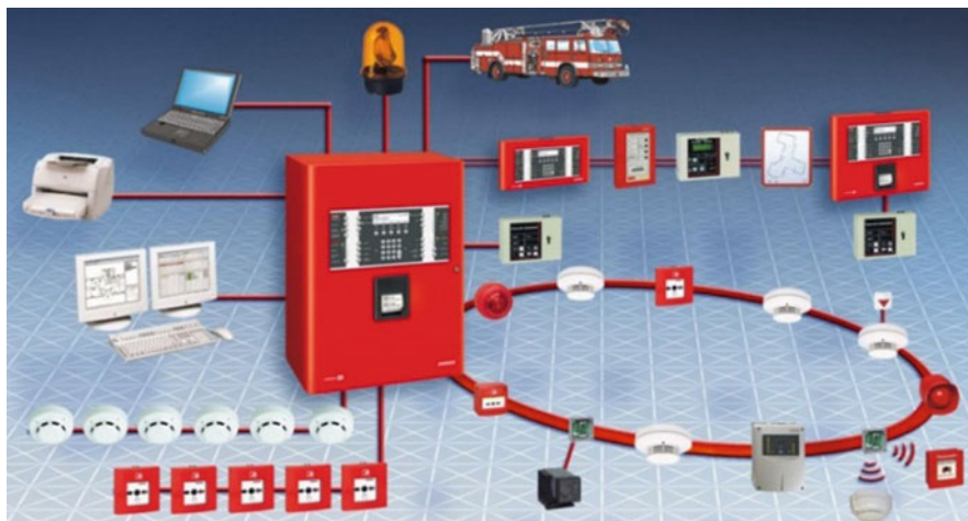
Fig. 10.1 Fire protection system for modern buildings [2]
