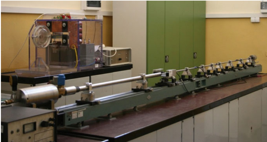
Fig. 10.6 Hopkinson Pressure Bar set-up for investigation of dynamic behavior of material [12]
