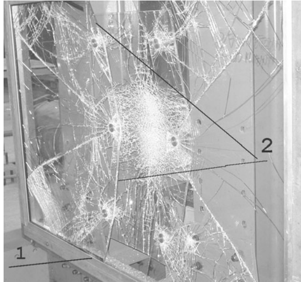
Fig. 18.9 The nature of cracking of the panes of the cash desk window following the fourth impact – view from the side where the load was applied. 1 – the pane ejected from the frame groove over the width of 140 mm, 2 – bending of the window panes
