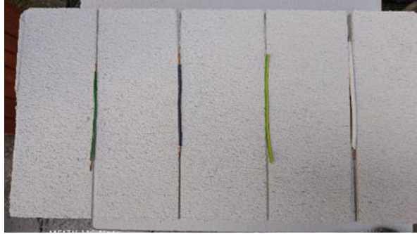
Fig. 23.2 Concrete brick prepared with cables without coating
