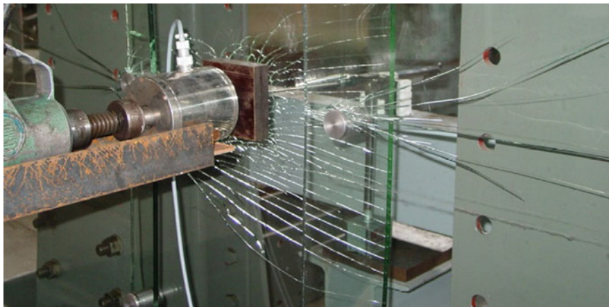
Fig. 18.6 Cracked panes of the cash desk window at maximum static load 2042 N – view from the side where the load was applied
