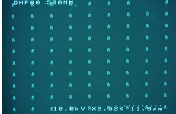
Fig. 19.9 Array of NCD nanopillars with a diameter of 500 nm
