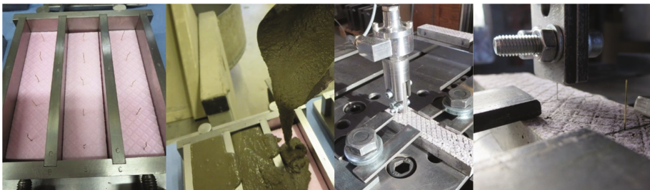
Fig. 1. Specimens preparation and configuration of the single fibre pull-out test.
