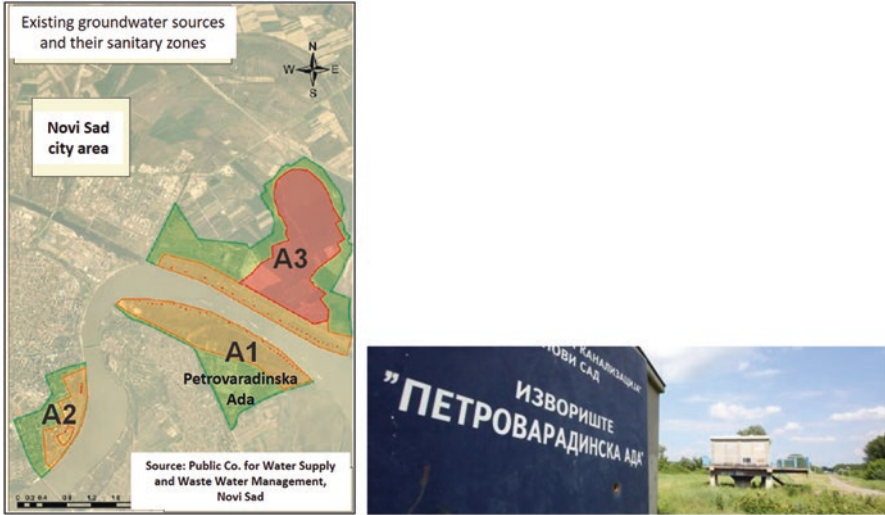
Fig. 23.4 Existing groundwater sources in Novi Sad with sanitary protection zones and Renney well at Perovaradinska Ada groundwater pond (A1)
