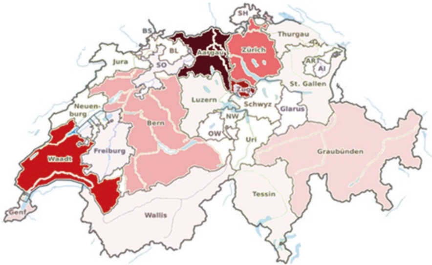
Fig. 6.3 The heat map of the cumulative economic losses at each canton of Switzerland due to propagation of cascading failures in the electric power system (Li et al. 2015)
