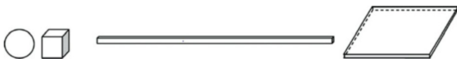
Fig. 23.17 Theoretical particulate shapes having the same volume equivalent diameter but very different external morphology [69].
