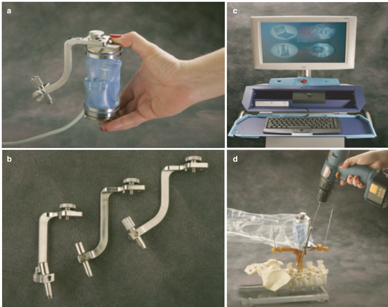
Fig. 17.20 SpineAssist. (a) SpineAssist device bone-mounted miniature robot. (b) SpineAssist workstation. (c) Three different types of arm (No. 1, 2, and 3 arms from the left). (d) Surgical setting of SpineAssist device for drilling
