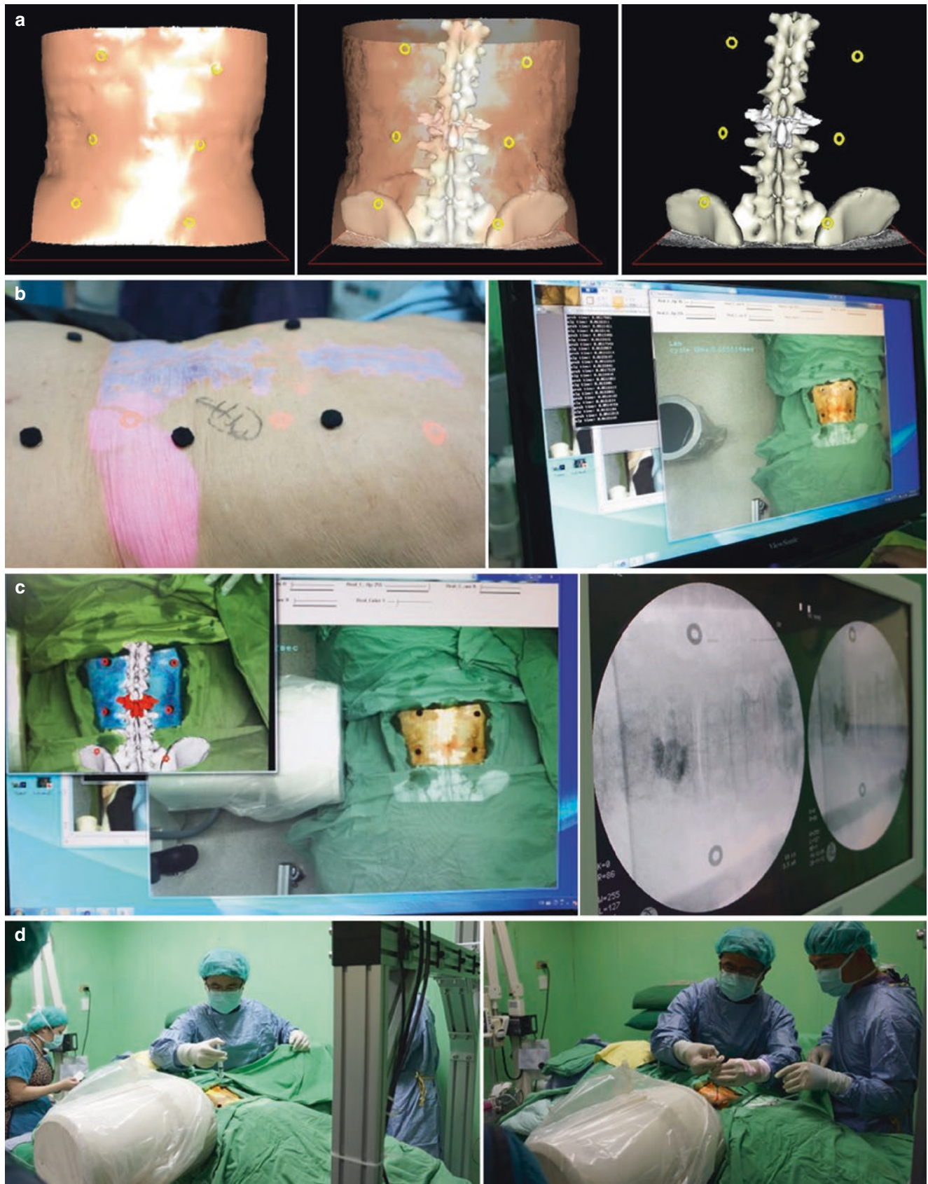
Fig. 15.13 The second clinical testing of the spinal surgery by using the proposed ARCASS system. (a) The 3D visible images of the patient which are generated by the visible patient tool. (b) The second patient experiment and the screenshot of our intraoperative software. (c) The
