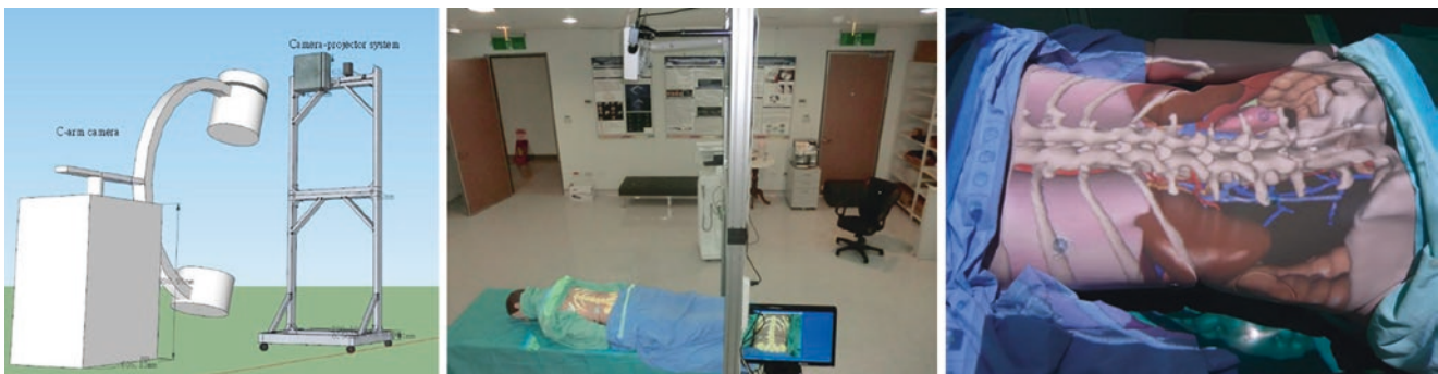
Fig. 15.9 The prototype of the proposed ARCASS system. A projector and an industrial camera are used for demonstration
