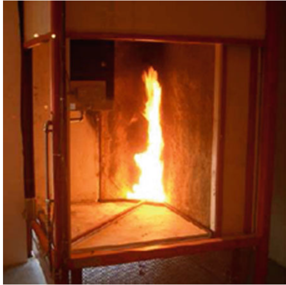
Fig. 7.1 Example of FBI test realized on straw wall coated with earth rendering [illustration (cd2e)]
