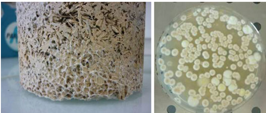
Fig. 8.10 Presence of fungi after conservation of hemp concrete at 30 °C and 98% RH (Hellebois et al. 2013)
