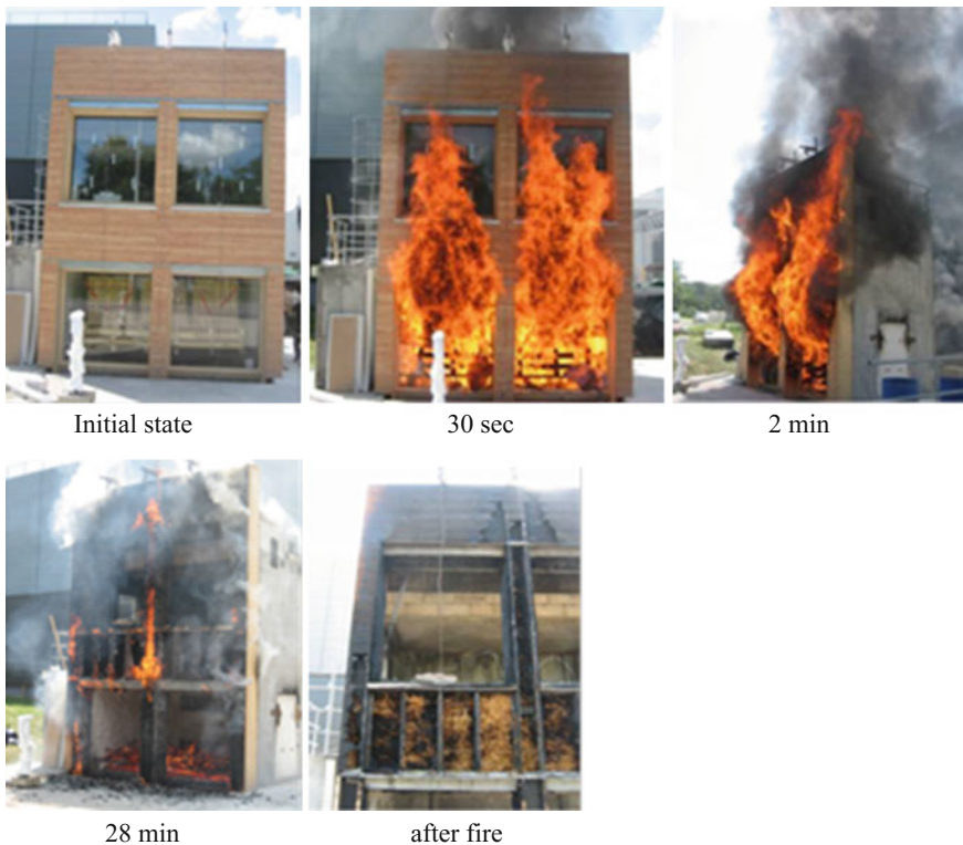
Fig. 7.7 Facade element made with wood and straw, test performed by CSTB (France) (CSTB 2009)
