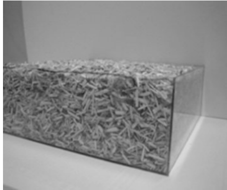
Figure 2 Hemp shiv placed in a PVC box
