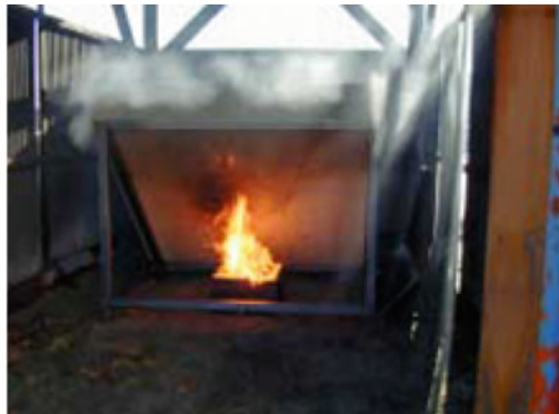
Roof element fire test (combustion of heptane)
