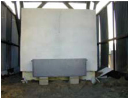
Straw wall : before fire test
