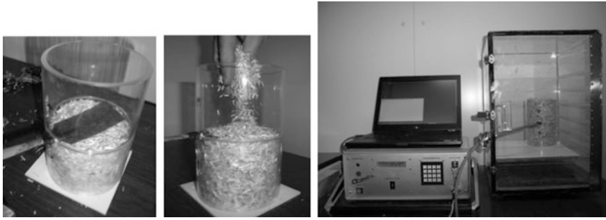
Figure 4 Measurement of thermal conductivity of hemp shiv (Lab F)
