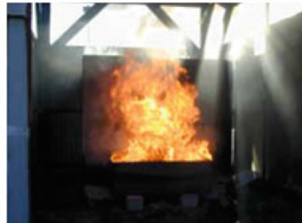
straw wall during fire test
