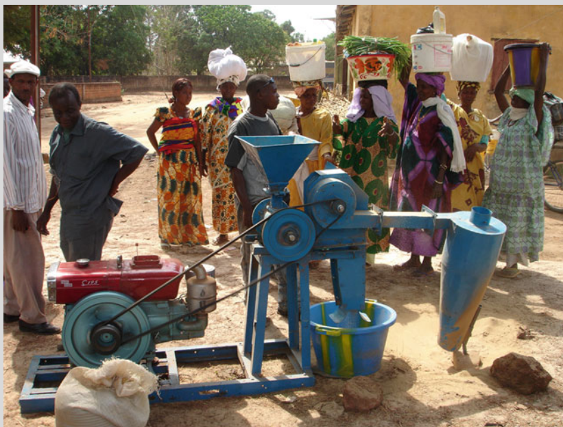
Fig. 12.1 Demonstrating the operation of the GMBF fonio huller in a village in Guinea (© Jean-François Cruz, CIRAD)
