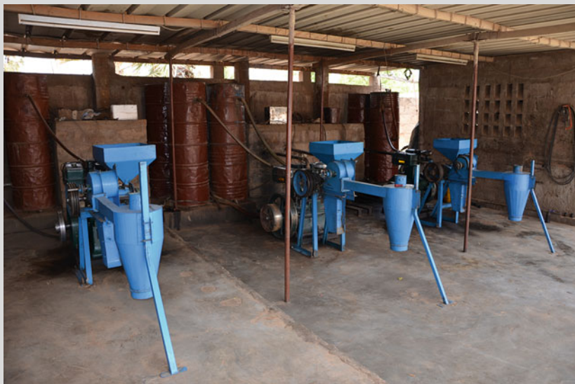
Fig. 12.2 GMBF fonio hullers in an enterprise in Burkina Faso (© Thierry Ferré, CIRAD)
