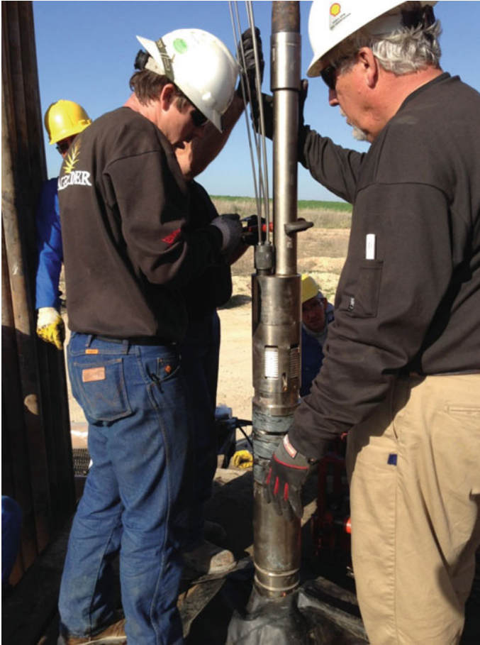
Fig. 8.8 D&L dual-mandrel hydraulic set packer with short string fitted with adapter to seal around control lines using compression fittings
