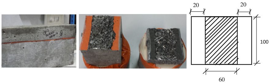
Fig. 3 Notched specimen for bond tensile strength test (dimensions are in mm)
