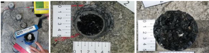
Fig. 3 Aspect of the portable equipment used in the pull-off test and tested sample
