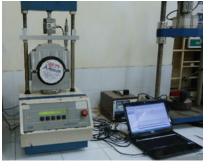
Fig. 1 Shear testing equipment and example of a test at 20 °C
