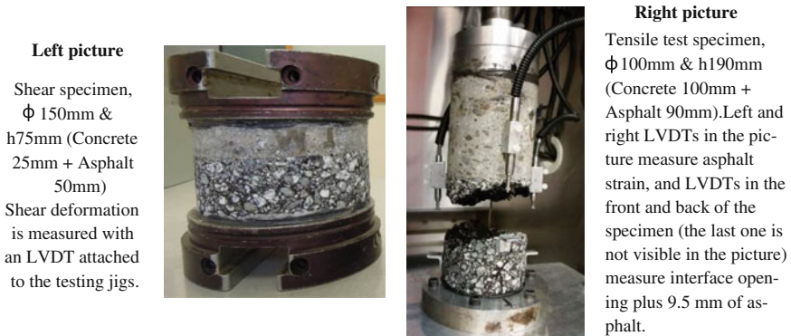
Fig. 1 SST ( left ) and UTM ( right ) composite specimens
