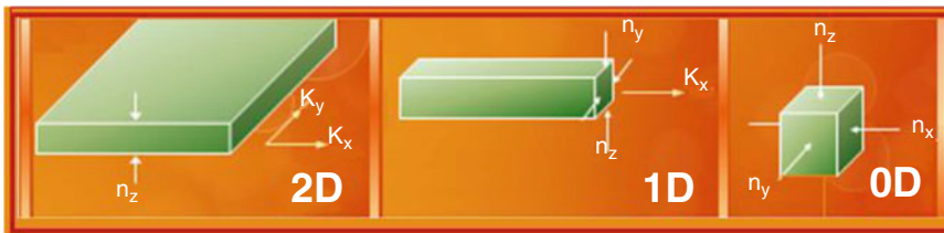
Fig. 3.4 Classification of the nanostructures based on the number of confinement spatial directions
