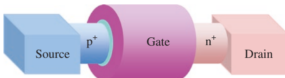
Fig. 17 Schematic diagram of a horizontal nanowire TFET structure
