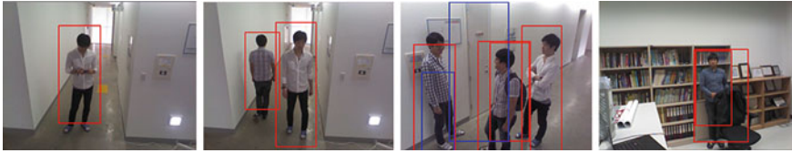
Fig. 13 Examples of human detection. Red boxes—true positives, blue boxes—false positives
