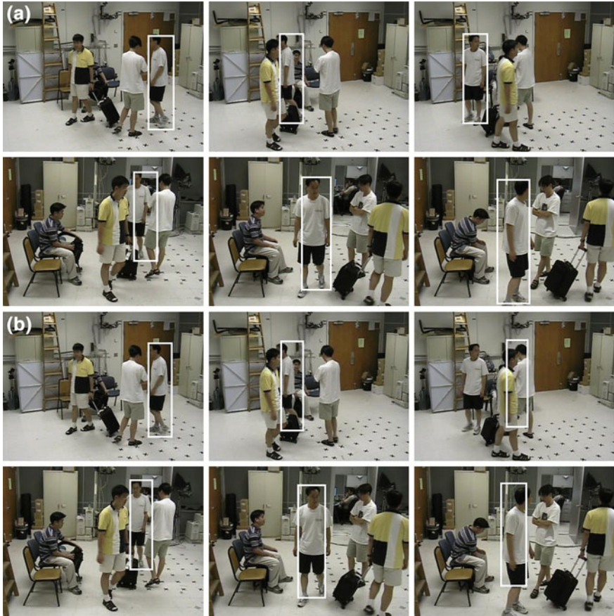
Fig. 5 Comparison between mixture KBF and conventional fusion by particle filter. The results at time t = 18, 54, 67 are presented for each algorithm in (a) and (b), where the first and second rows represent results in camera 1 and camera 2, respectively. Note that the target is lost after the second occlusions around t = 60 in (b). a Tracking by mixture KBF. b Tracking by conventional fusion method
