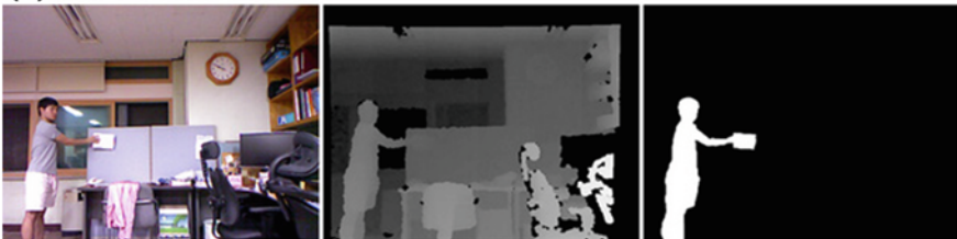
Fig. 3 Dataset samples of a color camouflage 1, b color camouflage 2, c normal situation, and d depth camouflage. For each situation ( a ), ( b ), ( c ) and ( d ), the color, depth and ground truth images are on the left , center , and right , respectively
