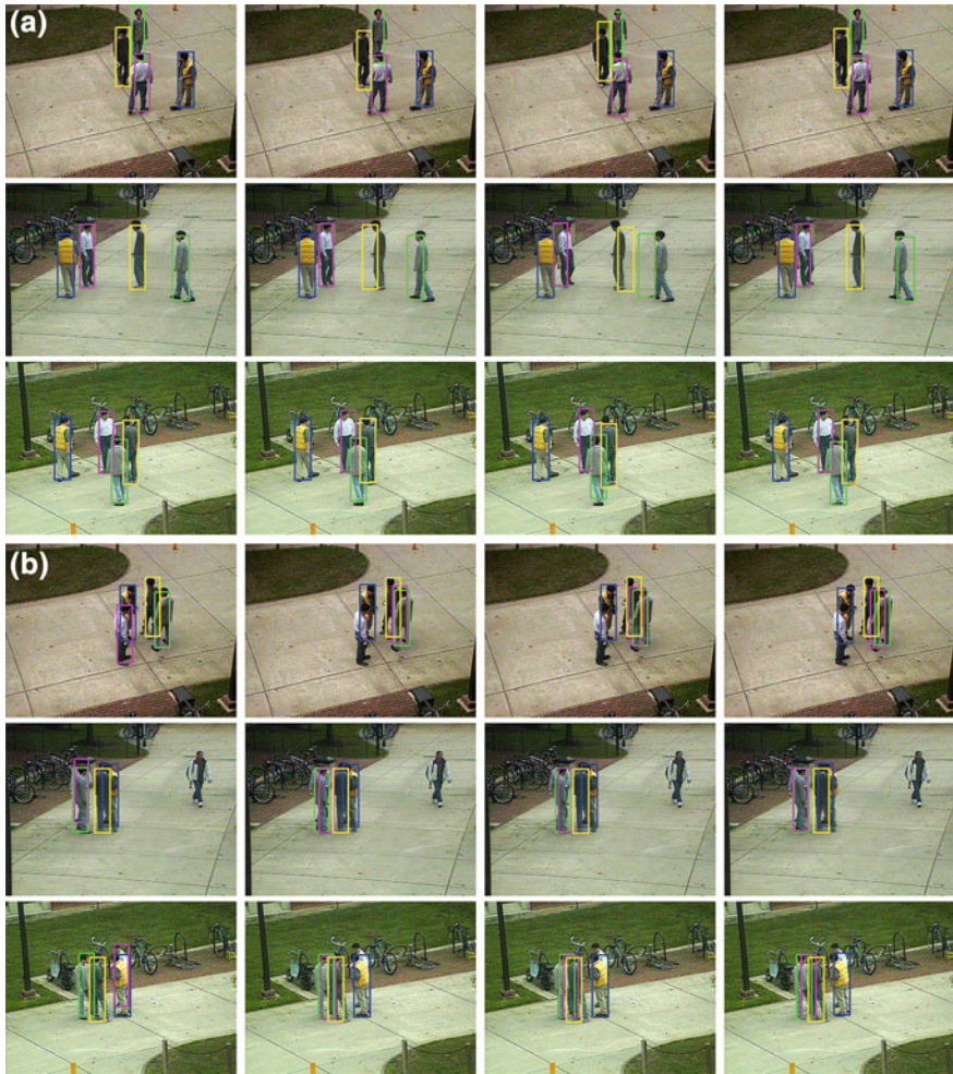
Fig. 7 Comparison of people tracking in presence of temporal sensor failures. (Col1) mKBF (Col2) KBF (Col3) PF (Col4) mKBF with even sample distribution. (Top) camera1 (Middle) camera2 (Bottom) camera 3. The errors are significant in person 2 (green) and 4 (yellow) at t = 529 and person 3 (magenta) at t = 685 . Note that the signal from camera 2 is completely noisy t = 529 but we presented a normal image to show tracking performance effectively. a Tracking results at t = 529 . b Tracking results at t = 685
