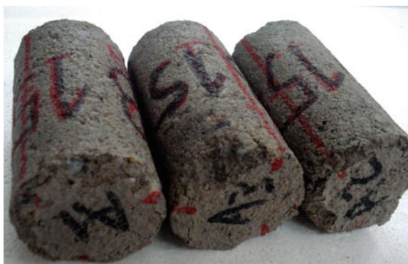
Fig. 3 Wear of the specimens due to intrusion of sulphates on the edges
