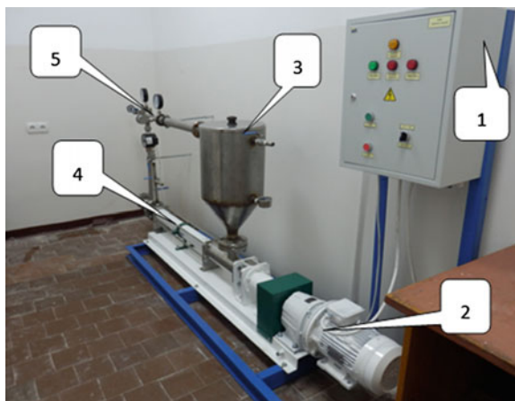
Fig. 1 Appearance hydrodynamic cavitator: 1—control panel; 2—motor-reducer; 3—reactor; 4—screw pump; 5—homogenizer
