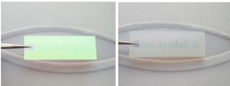
Fig. 6.27 Left , a colloidal photonic crystal deposited onto a microscope slide and held at the correct angle such that the camera catches the Bragg reflection. Right , the same sample after the slide has been tilted away from the Bragg reflection angle. Note that the transparency of the sample is partially restored simply by tilting
