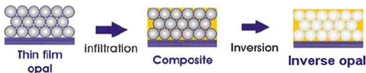
Fig. 6.15 A schematic representation of the infilling and subsequent inversion of a thin film colloidal photonic crystal, in this case an opaline structure (Adapted from Ref. [31] with the permission from IOP Science)
