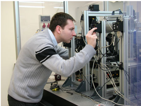
Fig. 4.4 Laboratory equipment for GISAXS analysis of nanoparticle arrays substituting to some extent the synchrotron beam facility (Institute of Physics SAS, Bratislava)
