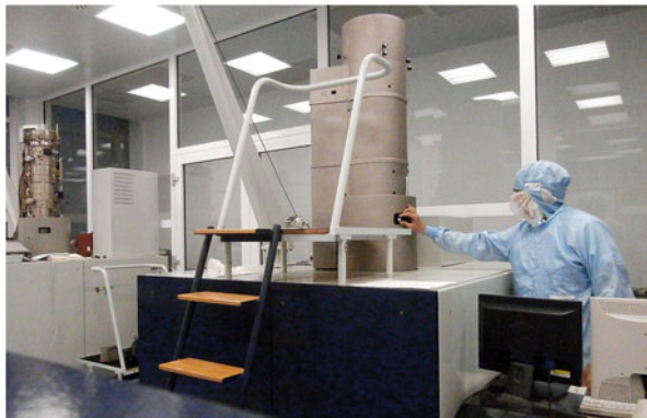
Fig. 4.5 Electron lithography apparatus in the clean room: air is maintained at well-controlled temperature and humidity level and it is filtered and circulated (With the courtesy of I. Kostič, Institute of Informatics SAS, Bratislava)
