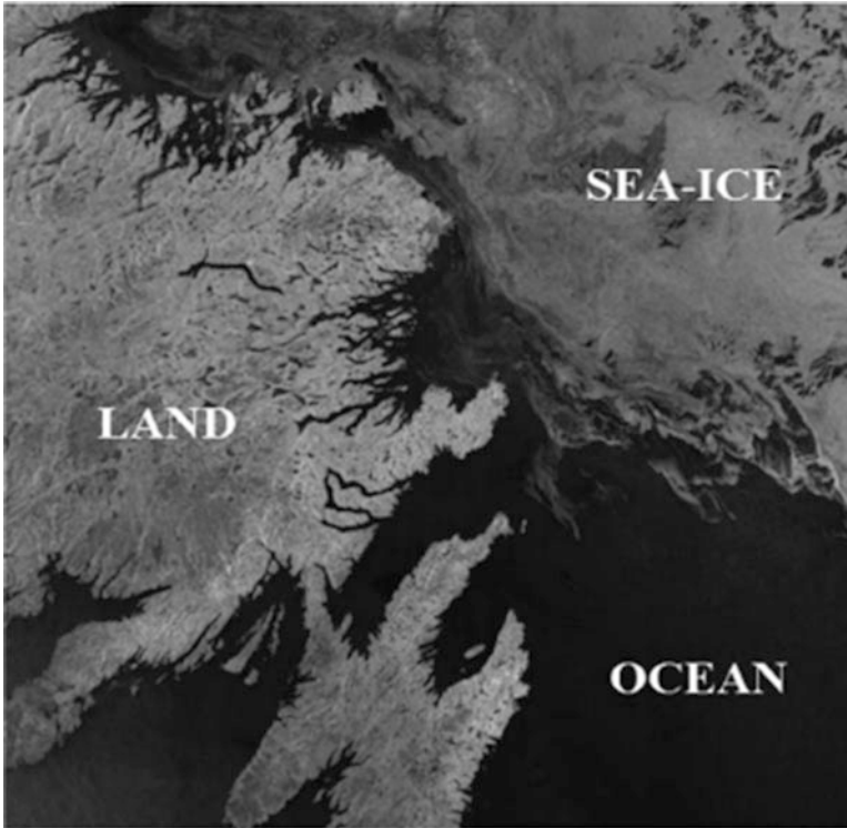
Fig. 6.5 RADARSAT-2 image ( 7,291 \times 7,296 pixels) covering the sea area nearby the Island of Newfoundland in Canada, ScanSAR Wide beam mode, HH polarization, taken at 22:29:36 on March 16, 2009
