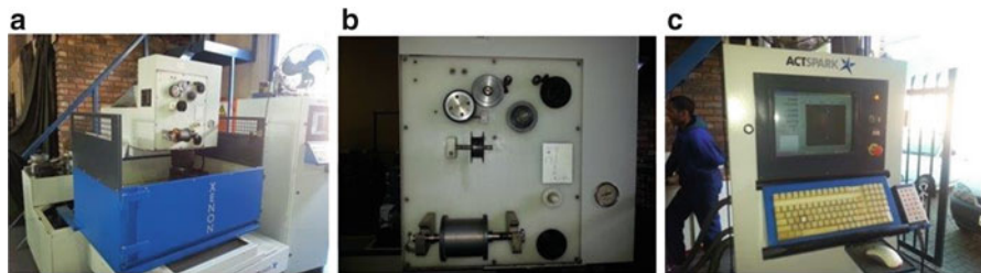
Fig. 10.4 WEDM system. (a) WEDM machine. (b) Wire reel. (c) Actspark control console
