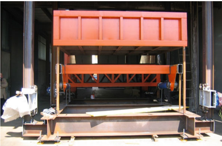
Fig. 9.8 Mechanical slope back view. The load cells are placed between part-A tank and its supporting frame. The cylinder placed between part-A and part-B can also be seen
