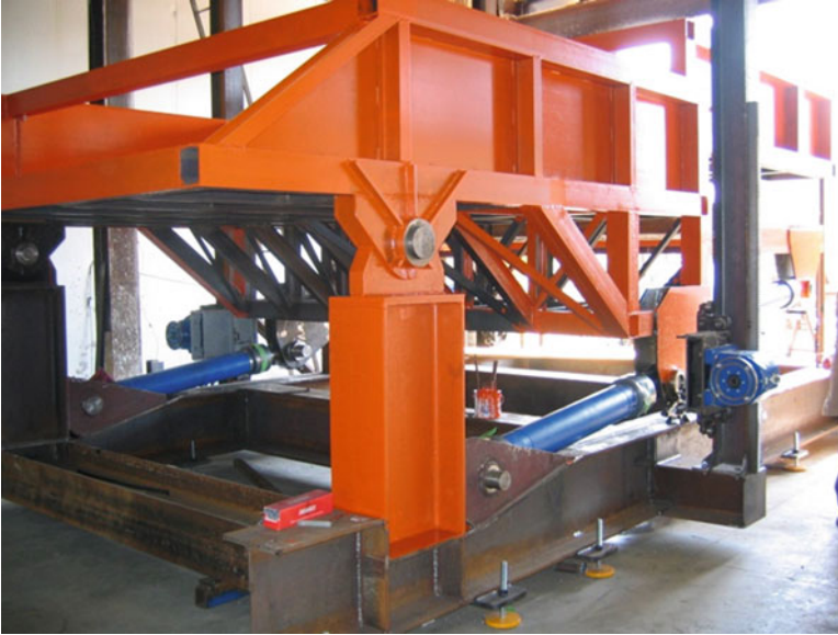
Fig. 9.7 Mechanical slope under construction: the connection between the base and part-B and the lower cylinders can be clearly distinguished. The base is supported by adjustable feet
