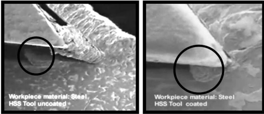
Fig. 28.1 Material build-up on the rake face of the cutting tip (BUE) (Amended from Balzers 2010)
