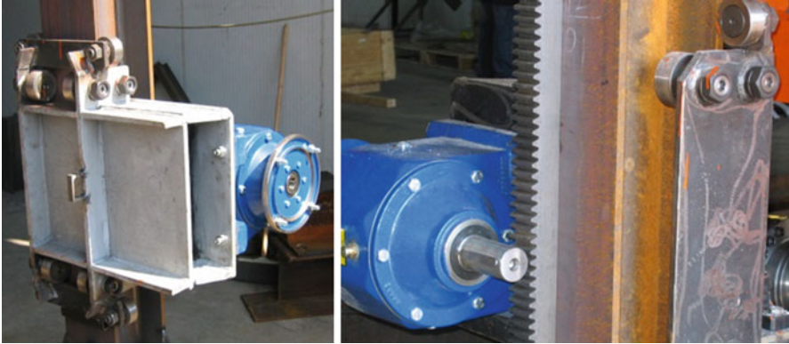
Fig. 9.9 The vertical slider allows the hopper to climb the column on which a toothed rack is welded (in the photo the gear-wheel is not yet spliced on the motor shaft)
