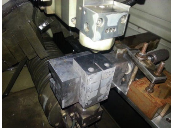
Fig. 10.5 WEDM of fatigue pre-crack
