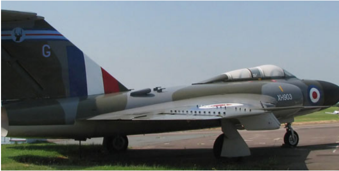
Fig. 6.37 Gloster Javelin FAW.9 with three rows of vortex generators on the wing to delay the onset of boundary layer separation. Photo Adrian Pingstone
