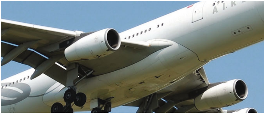
Fig. 6.52 Leading-edge fairing at the wing root of an A340-300 (photo A Pingstone)
