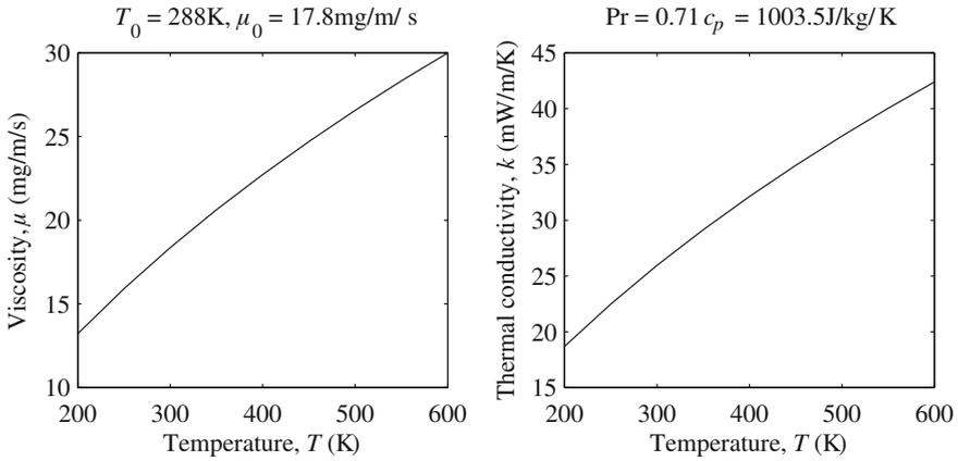
Fig. 2.8 Graphical representation of (2.81) and (2.82) for dry air
