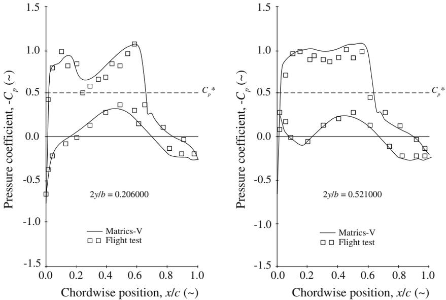
**Fig. 2.13** Comparison of predicted and measured pressure distributions about two sections of the Fokker 100 wing (from [20]). Note that this is a two-dimensional representation of results that were obtained from three-dimensional calculations (*Matrices-V*)
