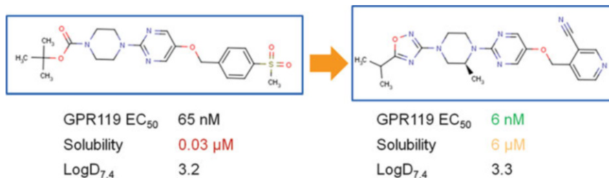
Fig. 9.3 Improvements to GPR119 agonists, following a strategy of introducing modifications that reduced the ‘self-complementarity’ of the molecule
