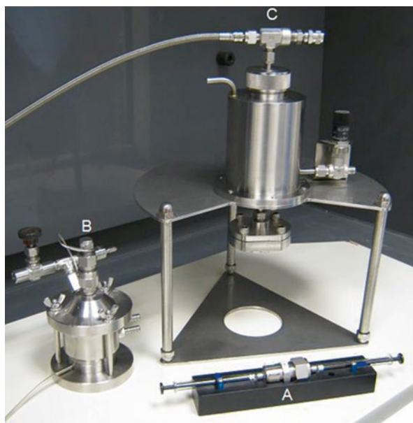
Fig. 26.1 Common types of research scale extruders used for producing liposomes. The mini-extruder (A) is a low cost option (Avanti Polar Lipids, Inc.) for producing small, under 1.0 ml, volumes and requires only manual pushes to drive the process. The high pressure extruders made of stainless steel (B and C) are driven by compressed gas. Extruder B (Lipix™, Northern Lipids Inc) is suitable for 1.0–10 ml scale while extruder C (Avestin Liposo-Fast™) has a 50 ml capacity. Both the latter devices have a thermobarrel for connection to a water circulating bath
