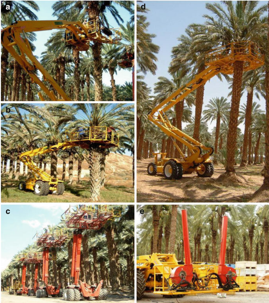
Fig. 8.6 High cranes used in date palm orchards in Israel. These machines are designed to work at various maximal heights of 11–20 m but can efficiently work also on shorter trees (b). They are either based on a flexible structure (a–b, d) or carry the platform on an extendable arm c. For the safety of the workers, the operator platform can conveniently approach the date below the crown (a) and then close to completely encircle the date tree trunk (b, d) to form a safe 360° working platform. Additional equipment, such as large bags for harvested fruit, hydraulic pruning tools, or mechanical sprayers (e), can be attached to these platforms and safely operated by the crew
