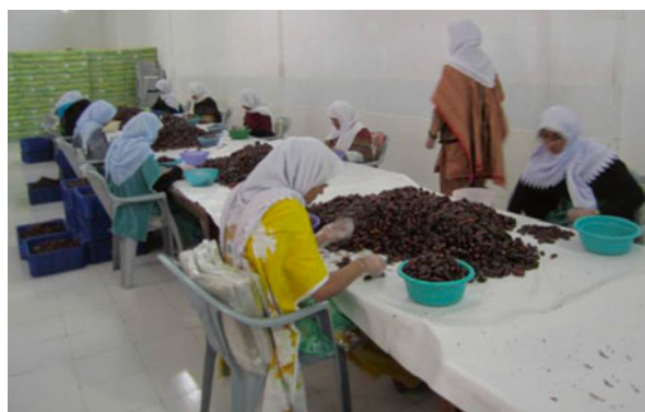
Fig. 5.31 Sorting the Rabai cv. dates into three categories according to size and freedom from blemishes
