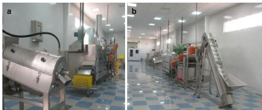
Fig 2.10 Date paste maker (a) and automatic washing and drying machine (b) in the first modern pilot date processing in Ahvaz, Iran
