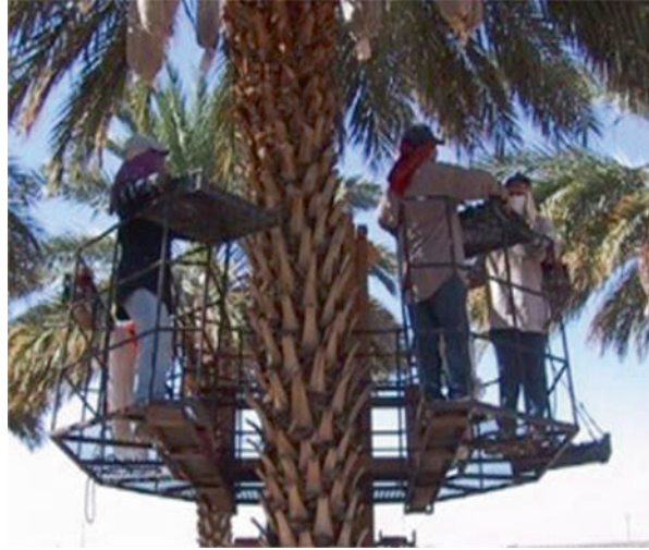
Fig. 6.17 Loaded U-Shaped harvesting platform (Source: Courtesy of H. Jayasuriya)
