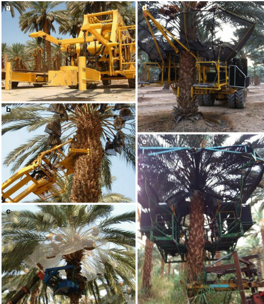
Fig. 8.7 Mechanical harvesters used in Medjool date palm orchards in Israel. The shaker units (a) are usually attached at the end of the high cranes, applying the shaking on the trunk close to its top, near the fruit bunches (b–d). Fruits can be collected in individual nets covering each bunch (b), in special nets below the entire crown surrounding the trunk of each tree (c), or in collection units attached to the platform of the high cranes, closing automatically around each tree crown, while shaking the trunk (d–e). Fruit can be transferred to picking trays on conveyors (d–e)
