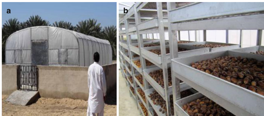
Fig. 5.25 The solar dryer (solar tunnel) unit. (a) The transparent plastic tunnel, (b) thirty stands inside the tunnel used for drying the unripe date fruit
