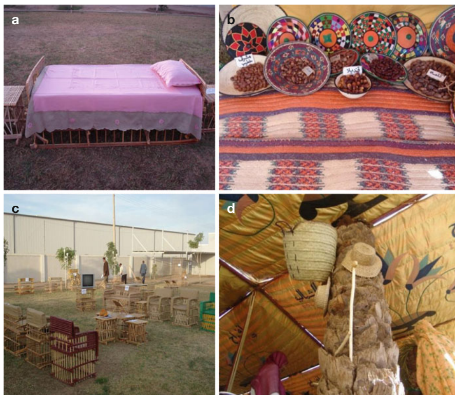
Fig 5.16 Manufacturing date palm parts. (a) Bed from leaf fronds, (b) mats and containers from leaflets, (c) furniture from leaf fronds, (d) basket and hats from palm leaflets
