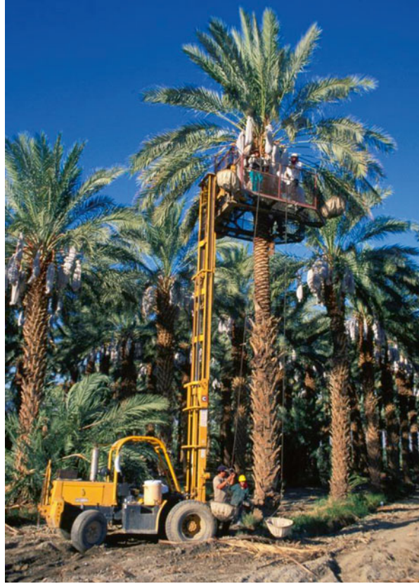
Fig. 14.2 Harvesting Medjool cv. dates using a mechanized lift and platform. Note mesh bags protecting fruit bunches (Photo by D. Karp)
