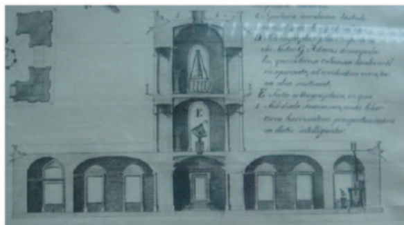
Fig. 7 Detail of the architectural plan of 1792 (Fig. 6), where we can see the instruments and its disposal on the OAUC building
